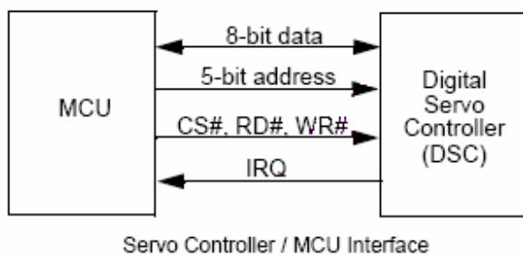
The digital servo includes an internal DSP, on-chip RAM and ROM, control logic, a loader interface, a serial interface, and an on-chip ADC-DAC, and interfaces with the MCU.
