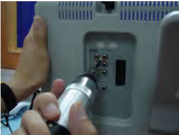
9. Remove the two screws fixed in rear casing.
